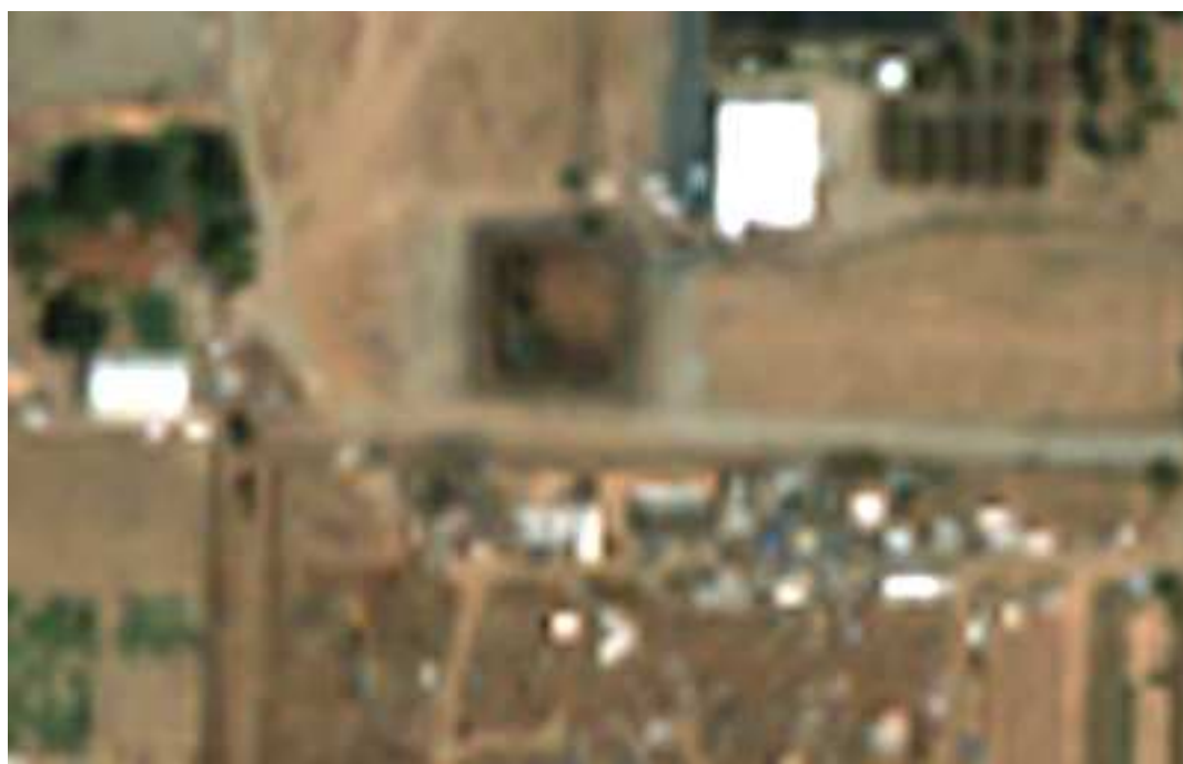
Fig. 6.16: Bicubic interpolation of the buildings region at zoom factor four.
