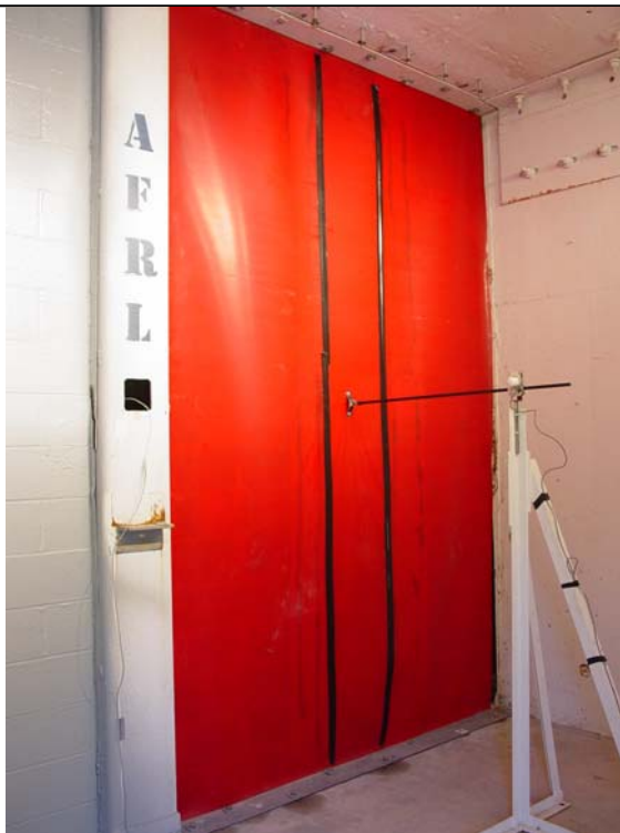
Figure 5.17 – CMU Wall with CUE Polymer Retrofit
