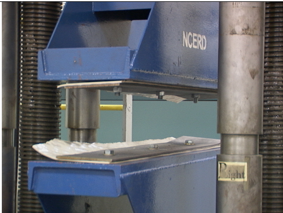
Figure 4.6 – Failure of Polymer Sample
