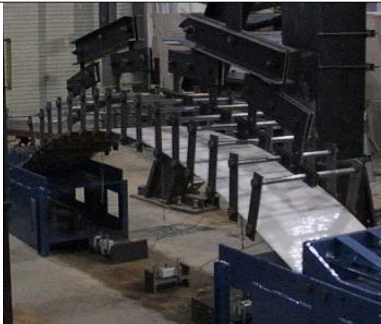
Figure 4.37c –Polymer Sample Nearing the End of the Test
