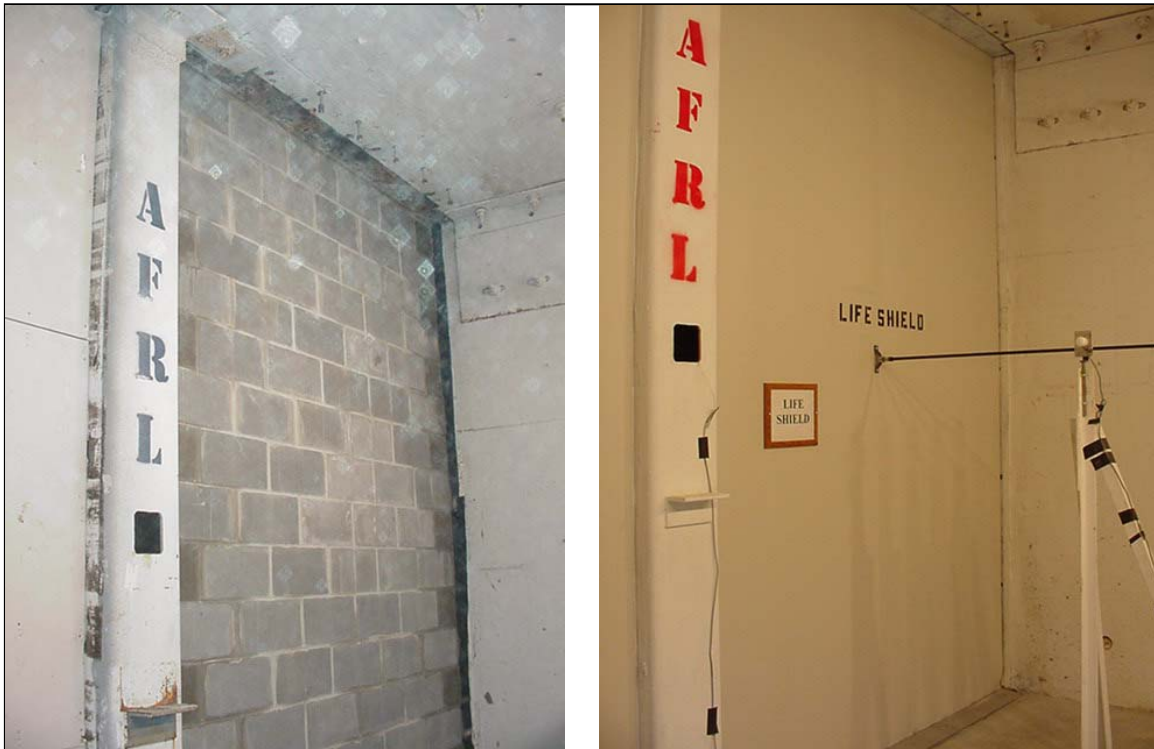
Figure 5.10 – CMU Wall with and without Polymer Sheet Retrofit
