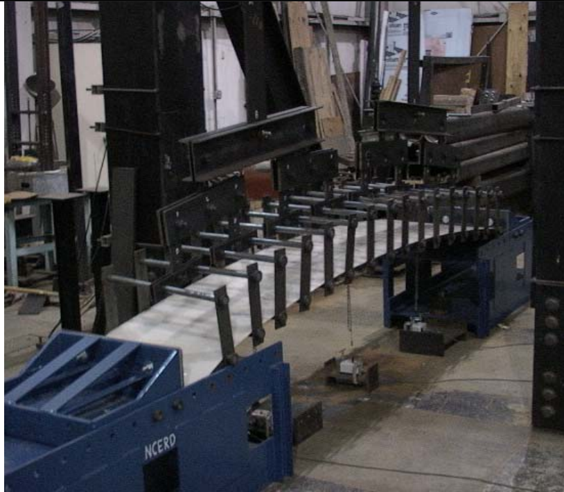
Figure 4.37b –Polymer Sample at the Beginning of the Test
