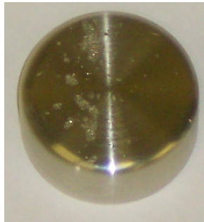
Figure 5-6. Photograph of the type 304 stainless steel electrodes following several hundred shots.
