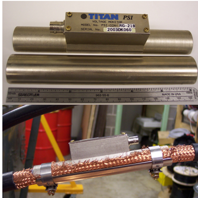
Figure 4-4. Photograph of the capacitive cable monitor prior to and following installation.
