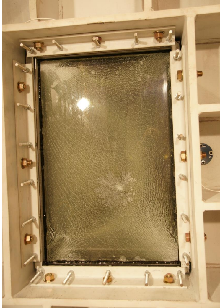
Figure 2.29 Laminated glass window panel was cracked after the GSA level E blast test. Both the outer surfaces of the glass plies were smooth to touch and minor damage to the composite interlayer
