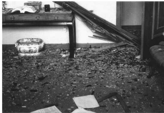
Figure 1.2 Glass fragments produced in Oklahoma City bombing (Reprinted with permission from “Survey of window glass broken by Oklahoma City bomb on April 19, 1995, revised”, copyright belongs to Glass Research and Testing Laboratory, Texas Tech University).
