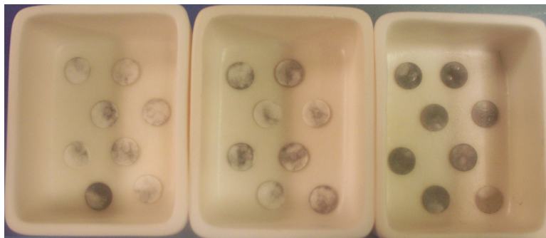
Figure 3.3: Contaminated chip dosimeters. It is hypothesized that increased surface area of particle processing creates an opportunity for moisture and other contaminants to adsorb onto the particle surface, which become trapped during pressing. Heating mixed powders in air at 350 °C improves pellet response homogeneity and eliminates greying (cf. figure 3.6).
