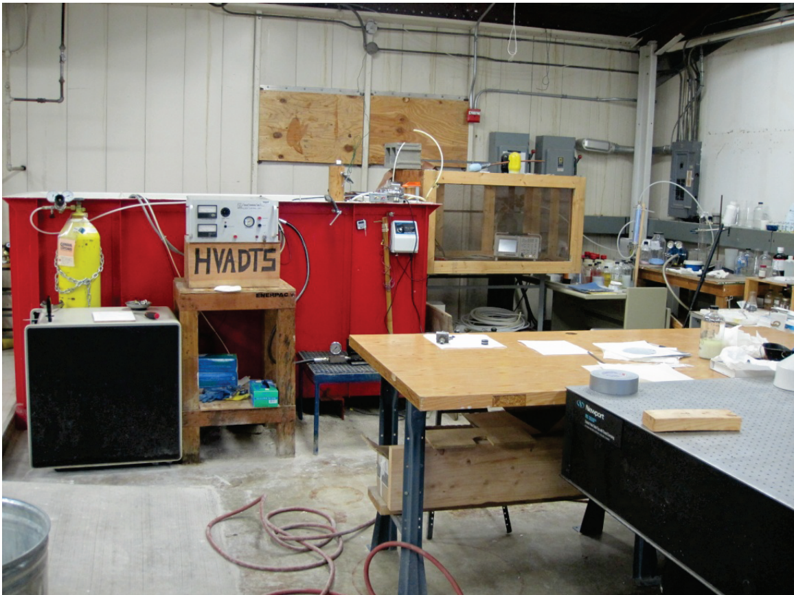
Figure 6.1: The HVADTS system is composed of a Marx Generator which drives a CLC circuit. The load consists of an oil switch in series with a 200 \Omega water resistor.
