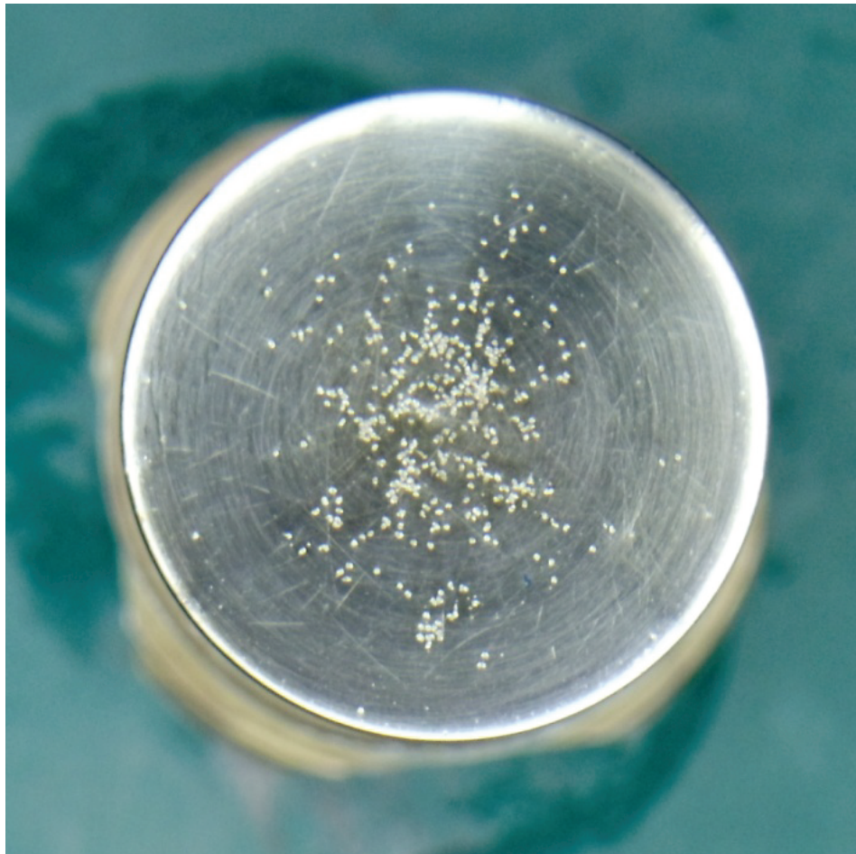
Figure 4.22: A previously smooth one inch diameter electrode is subjected to 230 breakdowns on the single-shot test stand. The deformations increase the probability that a subsequent breakdown will initiate on or near the site.
