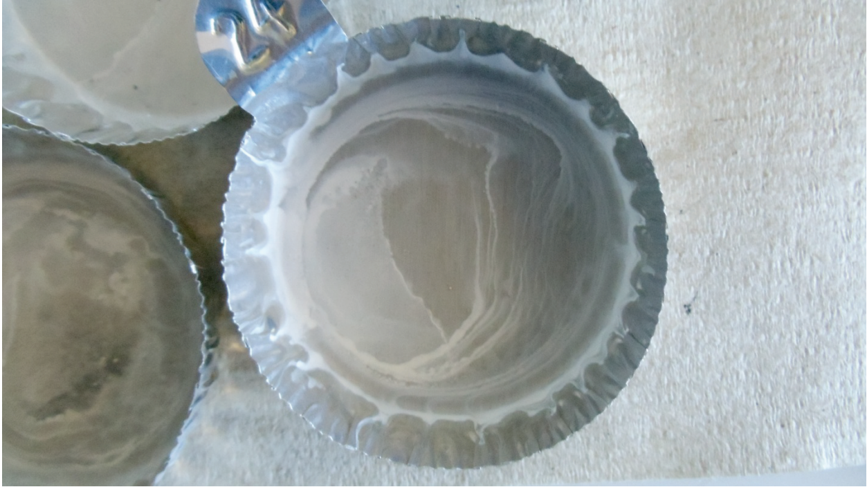
Figure 3.14: After the drying method all the oil is evaporated and only the BST particles remain.
