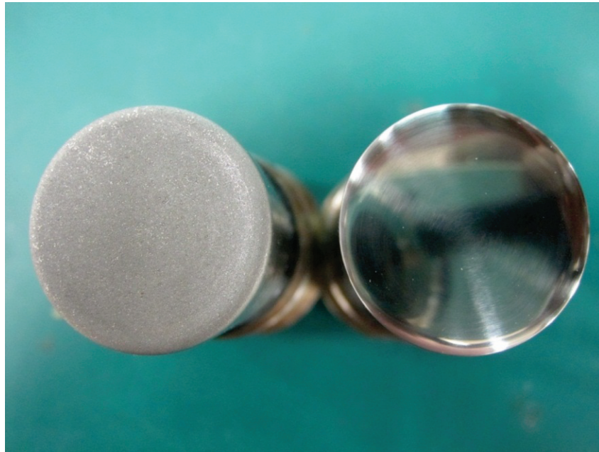
Figure 5.1: The two electrode surfaces utilized in the experimental analysis are the rough and smooth surfaces pictured. The rough surface (left) is generated with the use of sand-blasting and the smooth surface (right) is generated with 1200-grit sandpaper.
