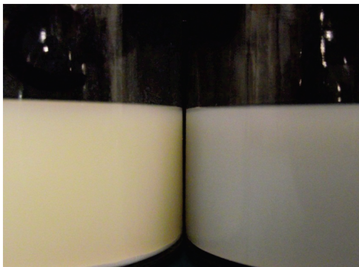
Figure 3.12: A photograph comparing the particle-infused Nycodiel PAO oil before testing (left) and after testing (right) demonstrates a strong carbon presence indicated by the darker color of the oil after testing.
