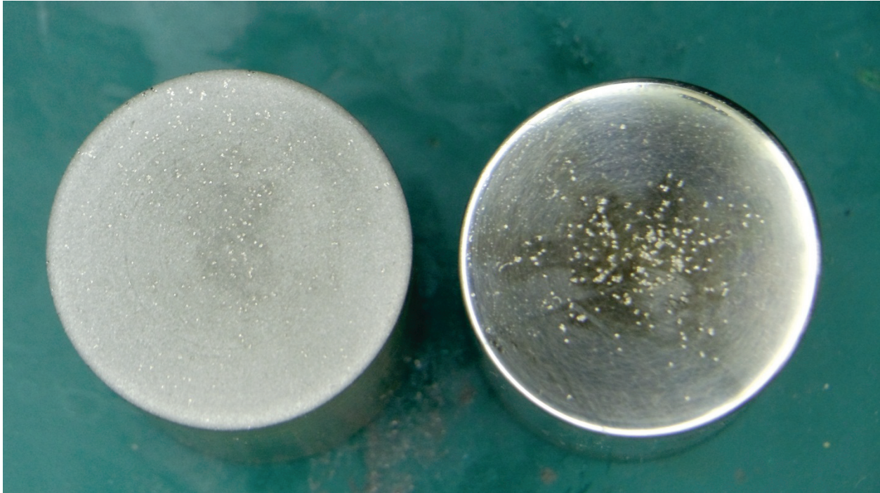
Figure 5.2: After 230 breakdowns, the rough and smooth electrode surfaces are pitted by breakdown arcs. The carbon on the surface is also a byproduct of the breakdown discharge.
