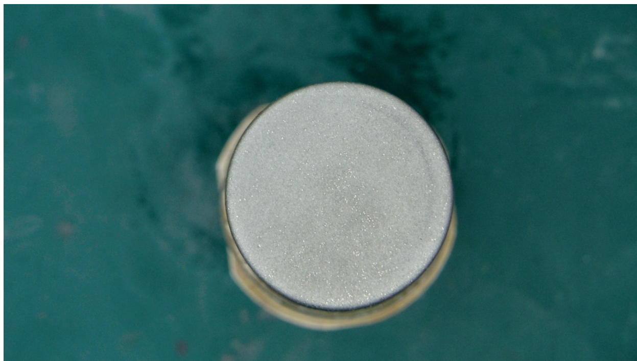
Figure 5.3: The rough electrode shows no trace of carbon after the acetone cleaning procedure. The electrode is ready to be reinstalled in the HVADTS system.
