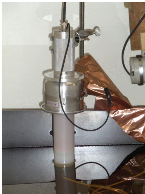
Figure 6.11: The Northstar Research PVM-6 100 kV, 80 MHz high voltage probe used to monitor the transient switch voltage.
