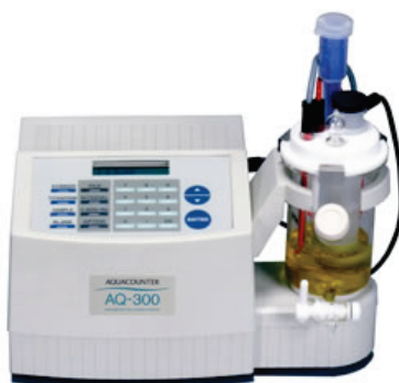
Figure 6.10: The JM Science Aqua Counter AQ-300 coulometric titrator used to perform water concentration analysis.
