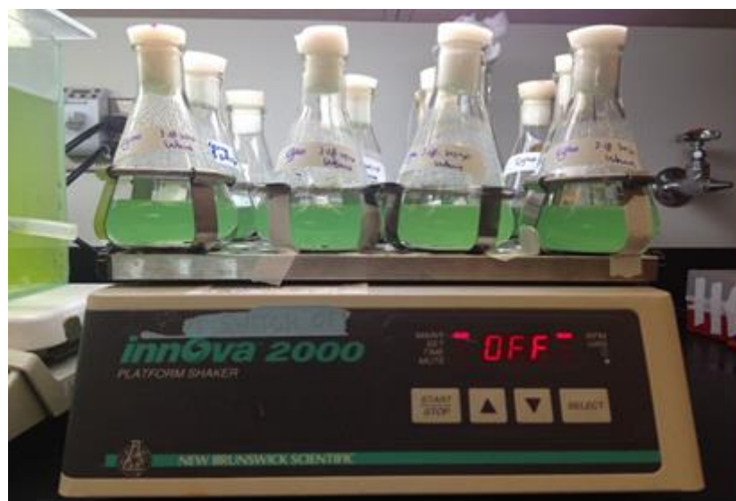
Figure 2.1 An experimental setup of batch study of phototrophic growth
