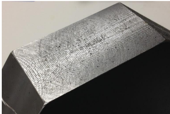
Figure A-6: Surface roughness specimen: medium profile finish
