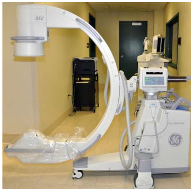
Minimally invasive fracture fixation is possible at the MU Veterinary Hospital because of the availability of an intraoperative fluoroscopy — a type of intraoperative X-ray machine, which allows for real-time imaging during surgery.
