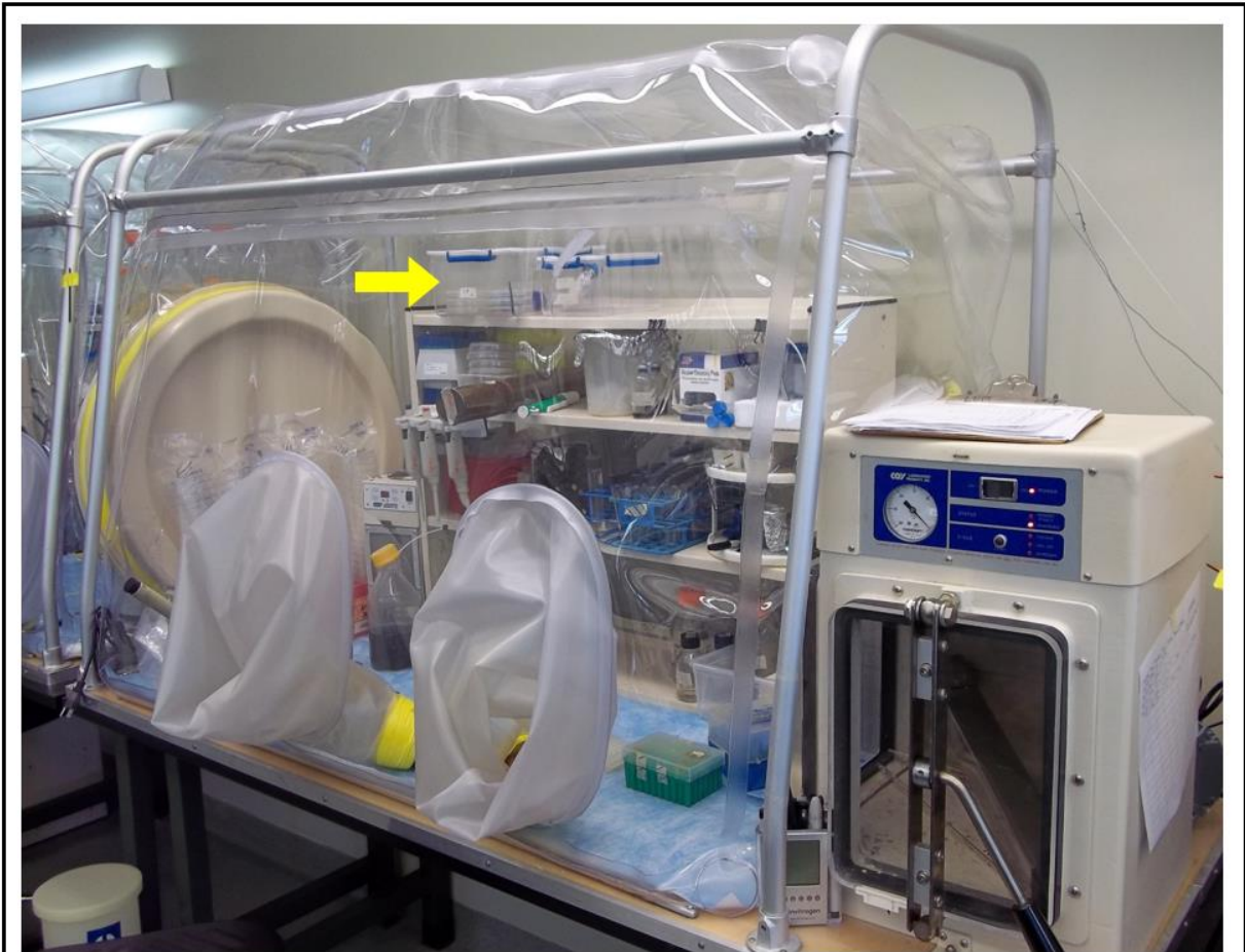
Figure 2. Anaerobic glove bag used for growth and manipulation of DvH. Smaller, sealed anaerobic boxes (arrow) are used for storage of plates containing growing colonies.
