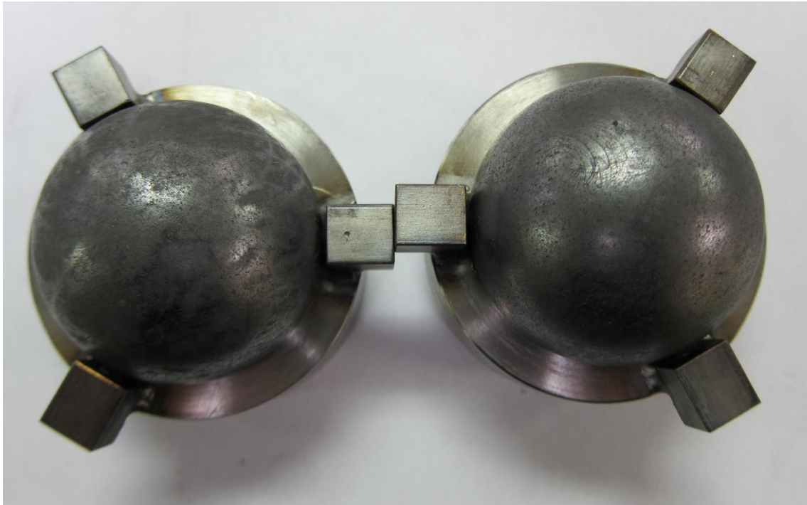
Figure 17. MLRF1 graphite mounted in sample holders before abrasion.
