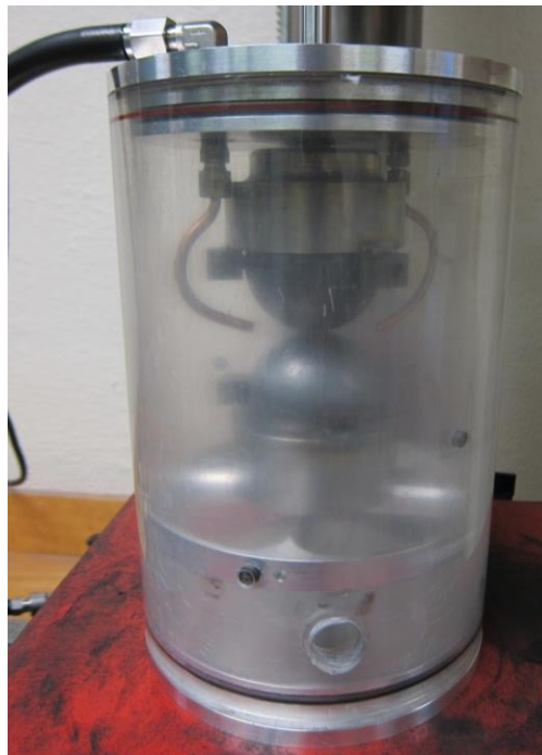
Figure 19. Picture of test chamber of MLRF1 graphite mounted.
