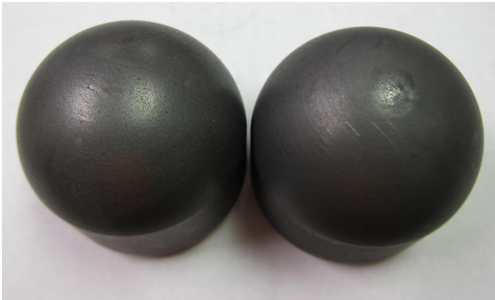
Figure 16. Commercial graphite samples mounted on sample holders before abrasion. This grade of commercial graphite was type GM-101 graphite obtained from Graphtek, LLC.
