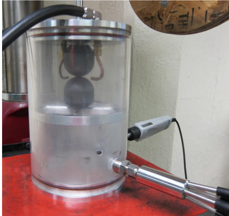
Figure 18. Picture of test chamber with commercial graphite mounted.
