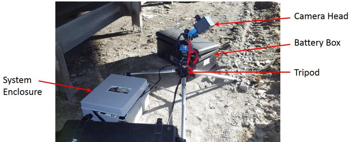
Figure 5-28: Setup for West Blvd. under I-70 in Columbia, MO
