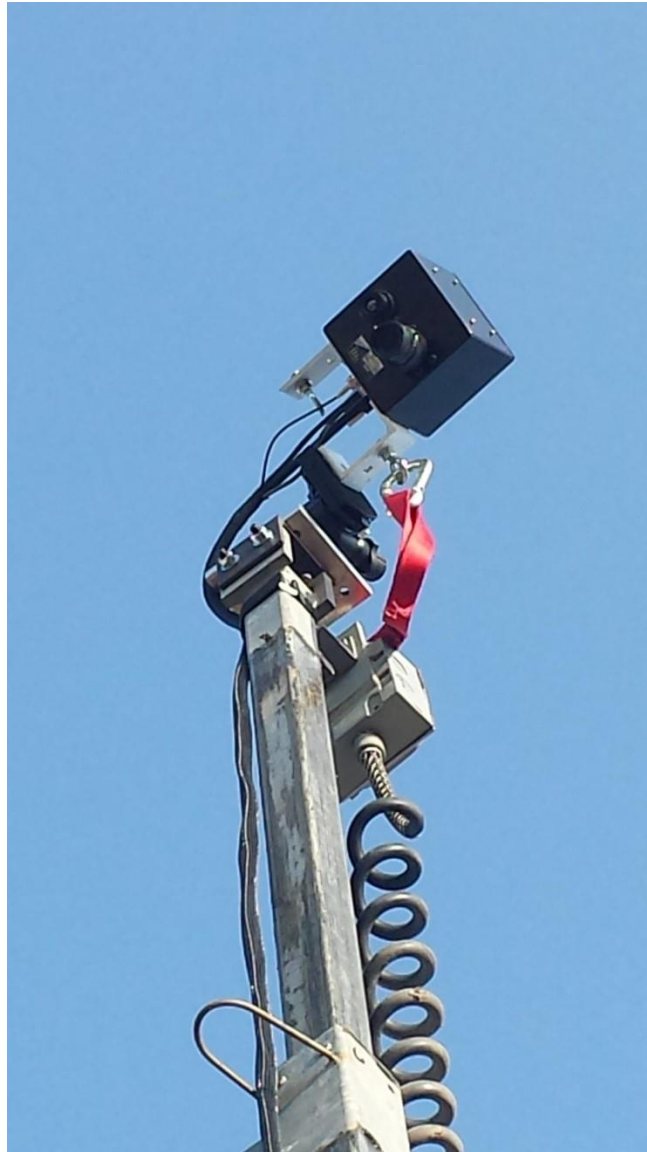
Figure 5-13: Camera head with lenses positioned in a vertical orientation
