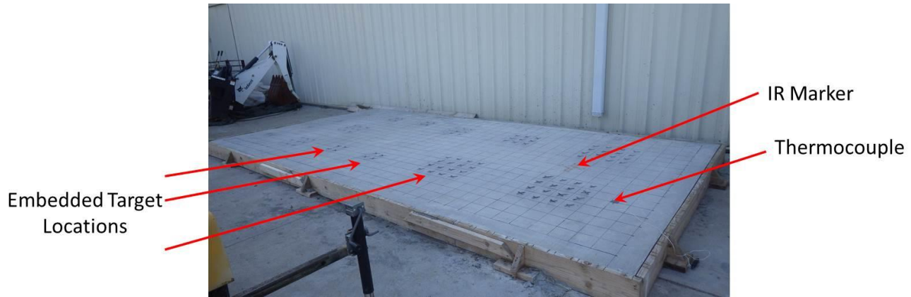
Figure 5-5: Concrete block constructed for testing nondestructive evaluation technologies
