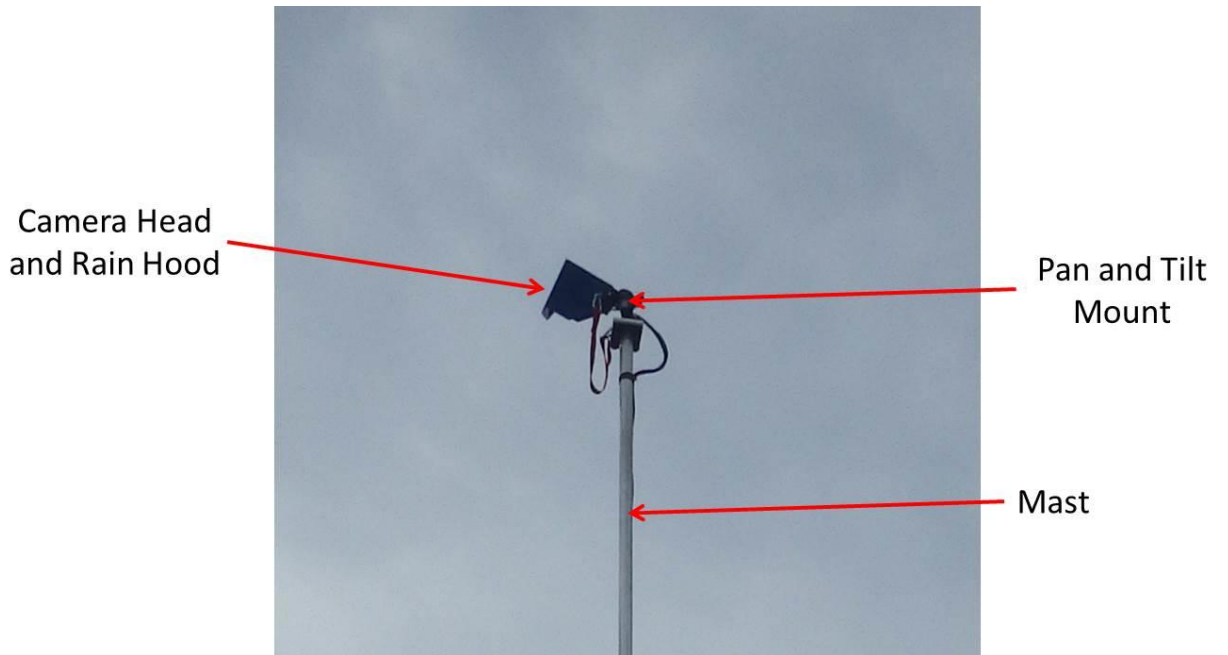
Figure 5-19: Close up of the pan and tilt mount and rain hood
