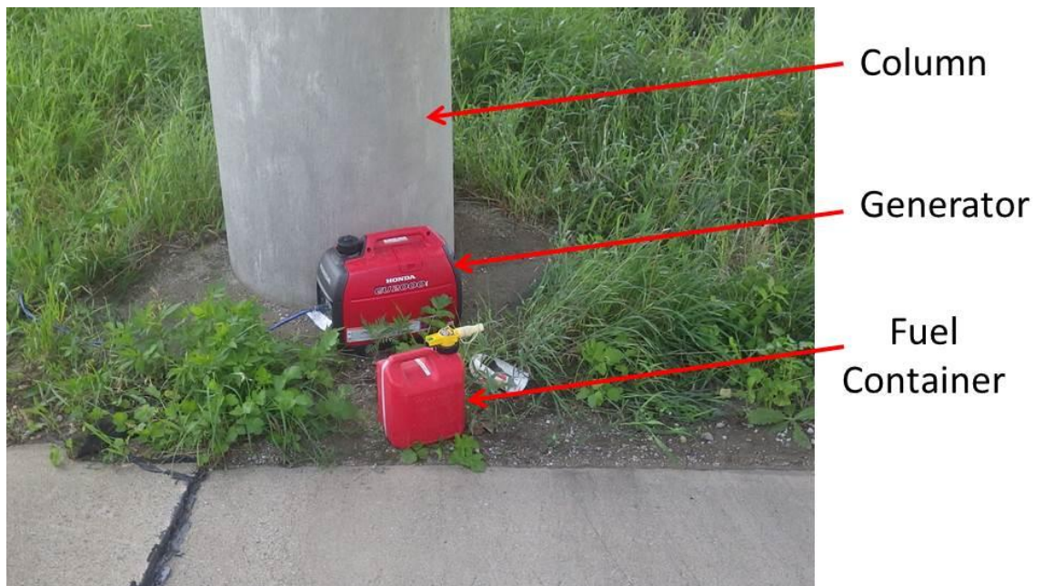
Figure 5-18: Generator used to power the IR-UTD system during the pretest
