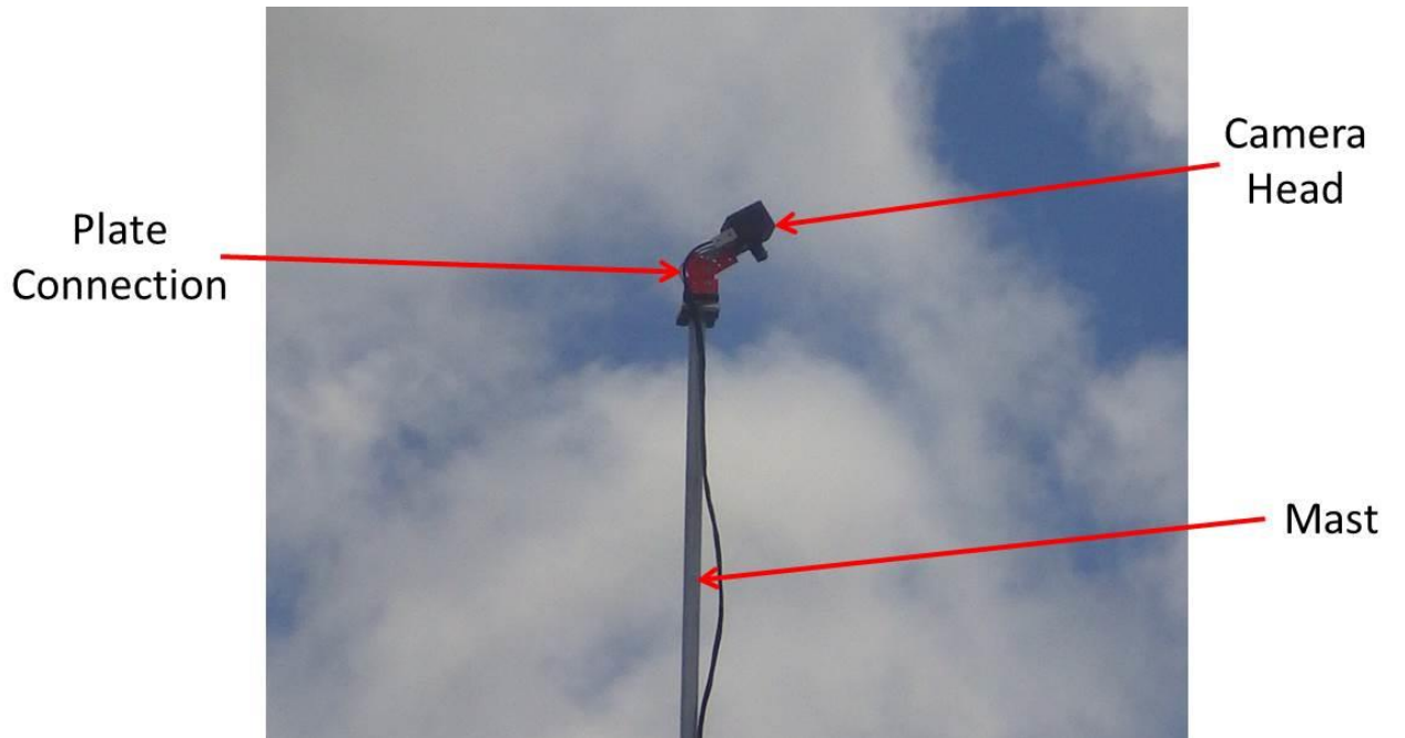
Figure 5-17: Close-up of the plate series used for mounting the camera head
