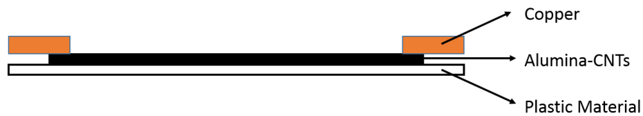
Fig 3.47 CNTs strain sensor fabricate outline process chart
