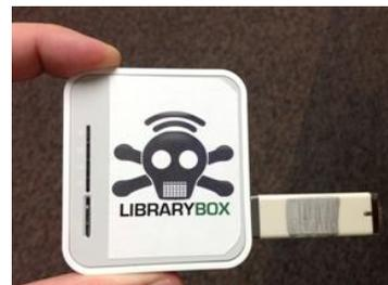
LibraryBox is a small, self-contained, portable download-only digital library. Consisting of a wireless hotspot (router), a flash drive,
