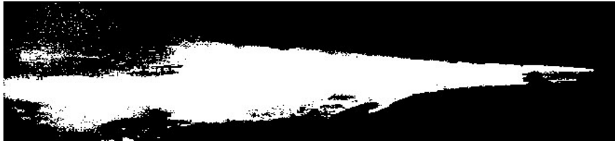
Figure 3.9 Incorrect Mask Due to Glowing Furnace's Interior Wall using Green Channel
