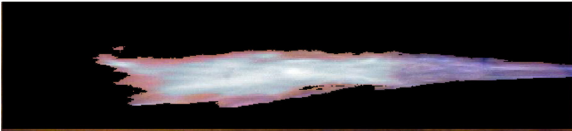
Figure 3.6 Masked Image based on Segmentation Mask derived from the Blue Channel
