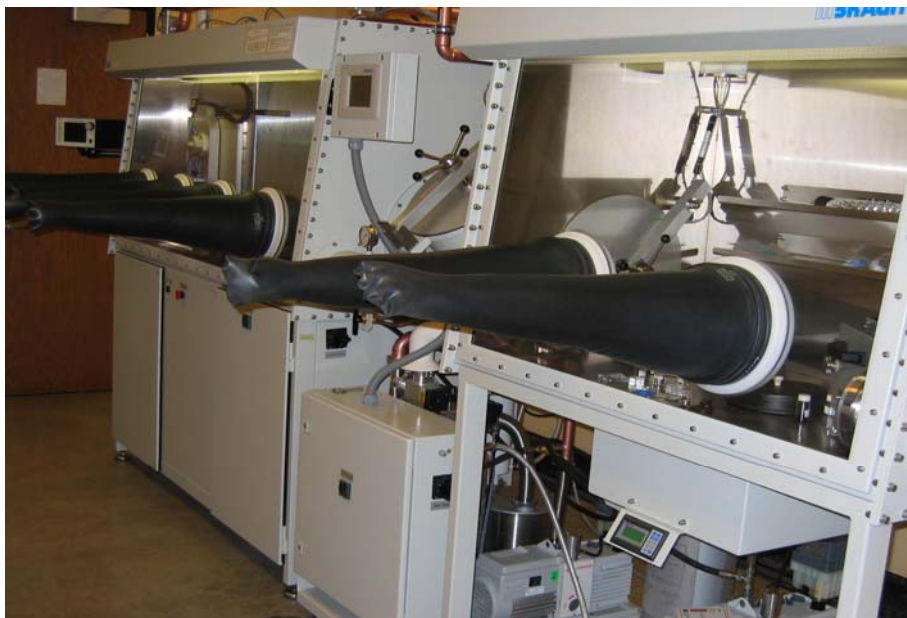
Figure (3.13): MBraun Glove box system with box A and box B.
