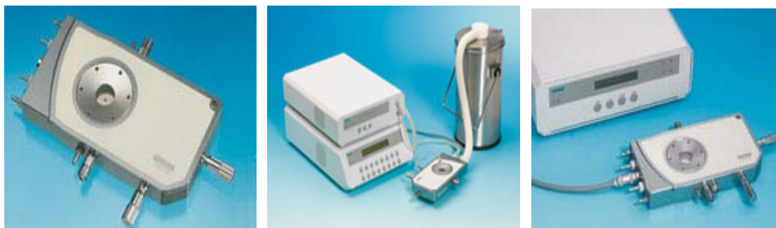
Figure (3.10): Linkam LTS 350 temperature stage and the temperature controller. 5
