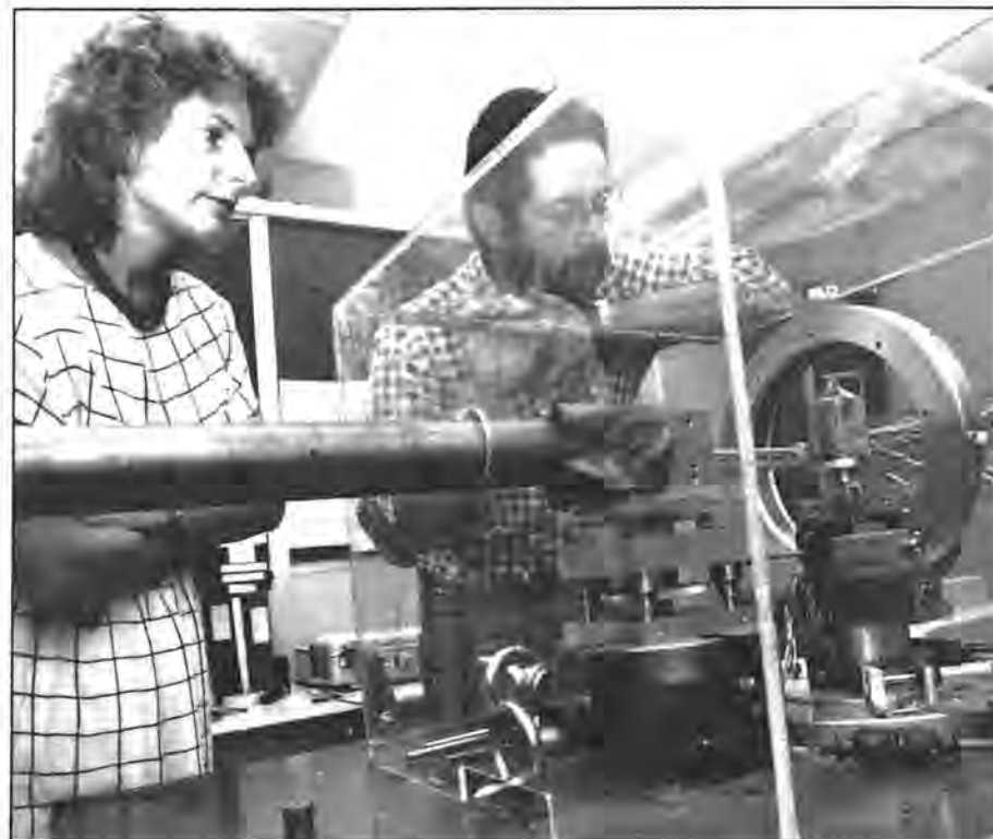
Wayne Pearson, a UMC graduate student, and Carol Ortale, a representative of the private firm that contracted with NASA to grow a mercuric iodide crystal in space, are shown with the encasement of the crystal. The crystal is about the size of a sugar cube.
