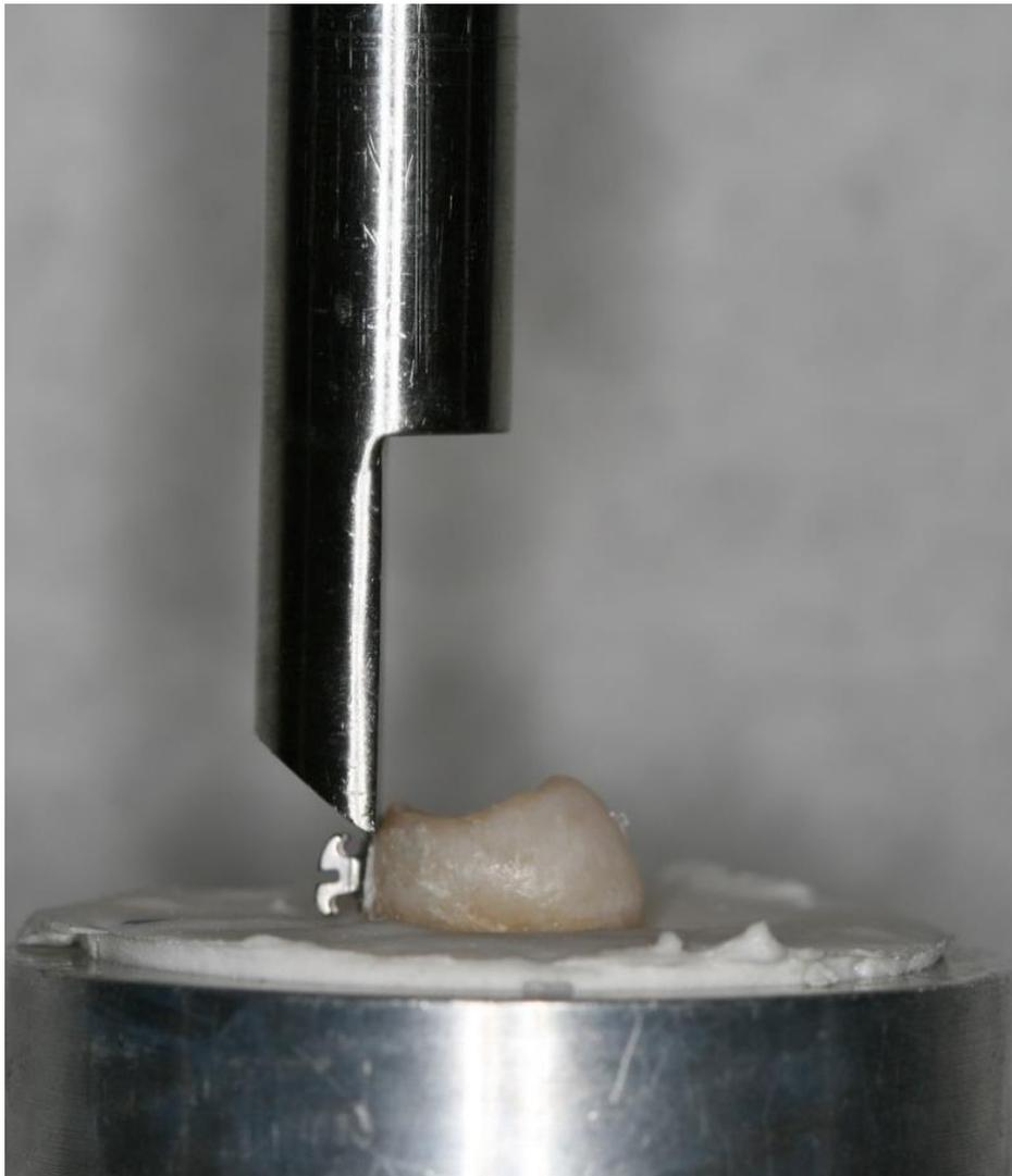
Figure 4. Bonded, mounted tooth ready for shear bond strength testing.
