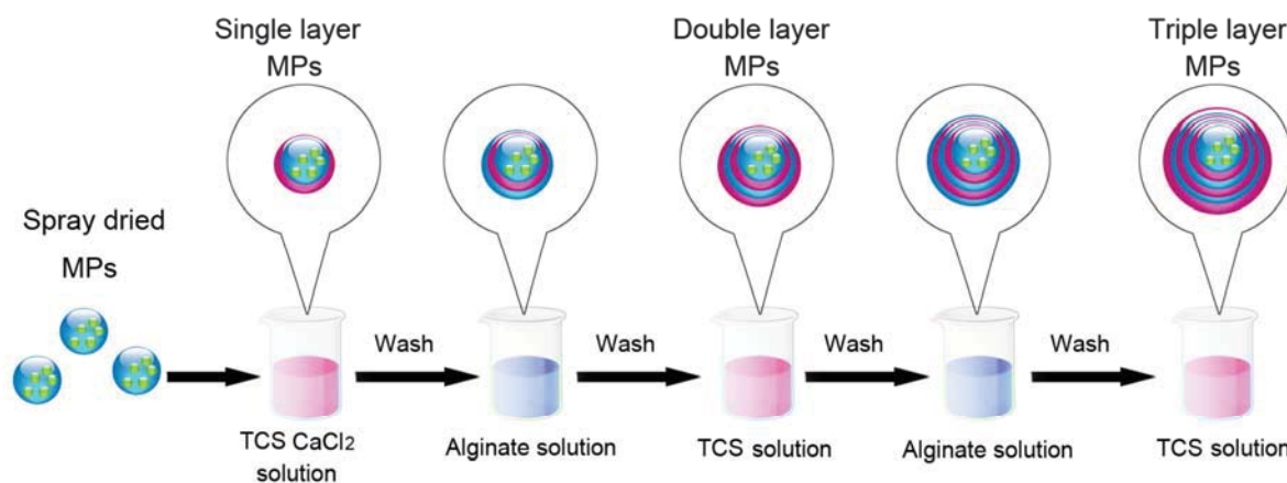
Fig. 5-1 Schematic preparation scheme of the TCS coated multilayer MPs.
