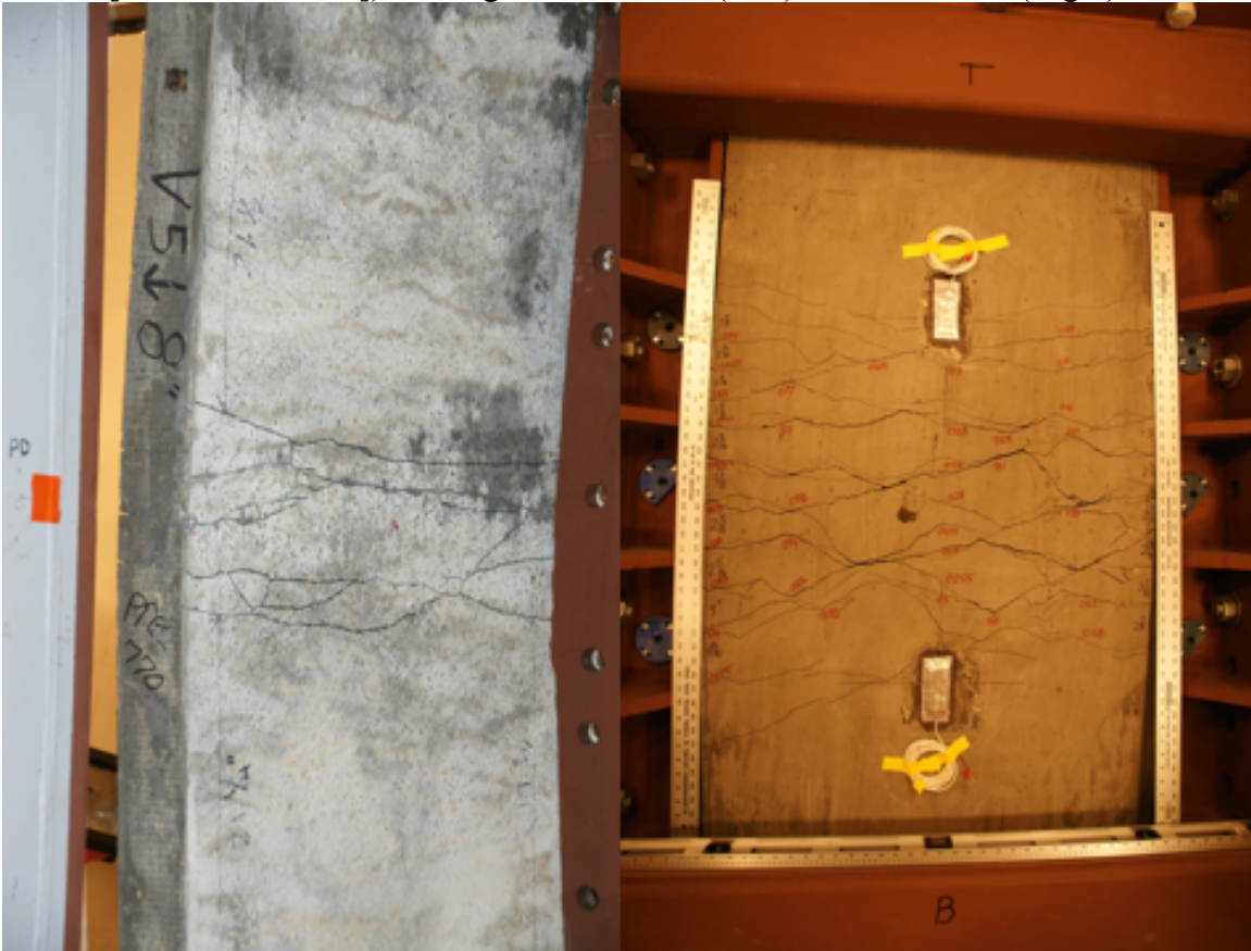
Figure 30- Damage to HSCV4 (8 in. [203.2 mm] Spacing; P = 41.1 psi [283.4 kPa]; I = 753.9 psi-msec [5198.0 kPa-msec]). Damage to Blast Face (Left) and Back Face (Right).
