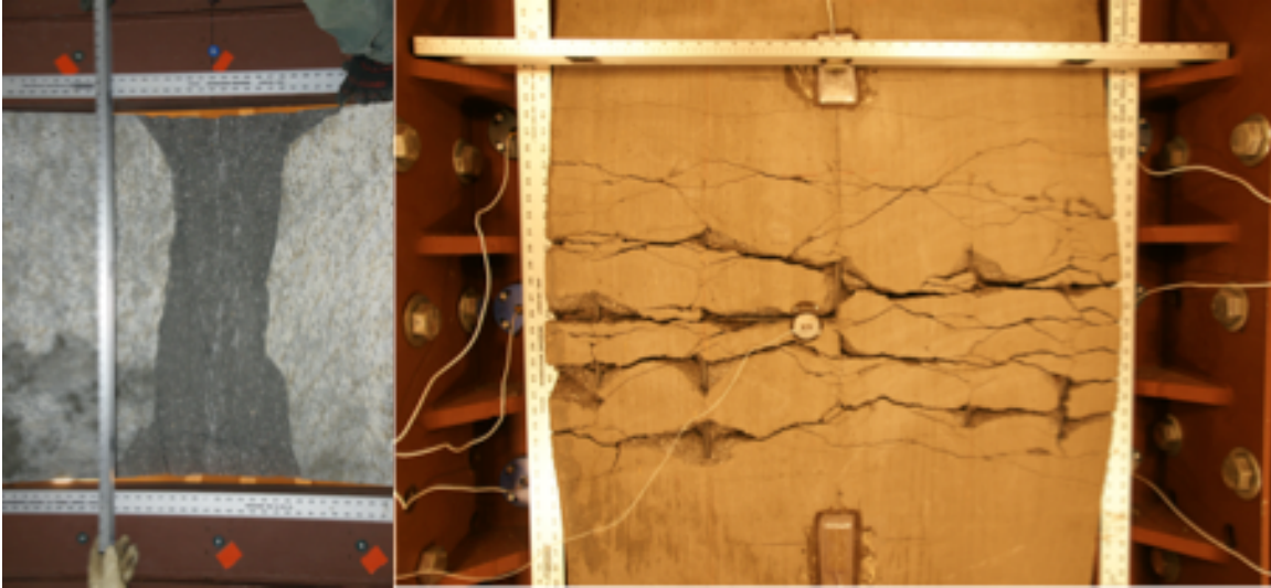
Figure 30- Damage to HSCV4 (8 in. [203.2 mm] Spacing; P = 41.1 psi [283.4 kPa]; I = 753.9 psi-msec [5198.0 kPa-msec]). Damage to Blast Face (Left) and Back Face (Right).
