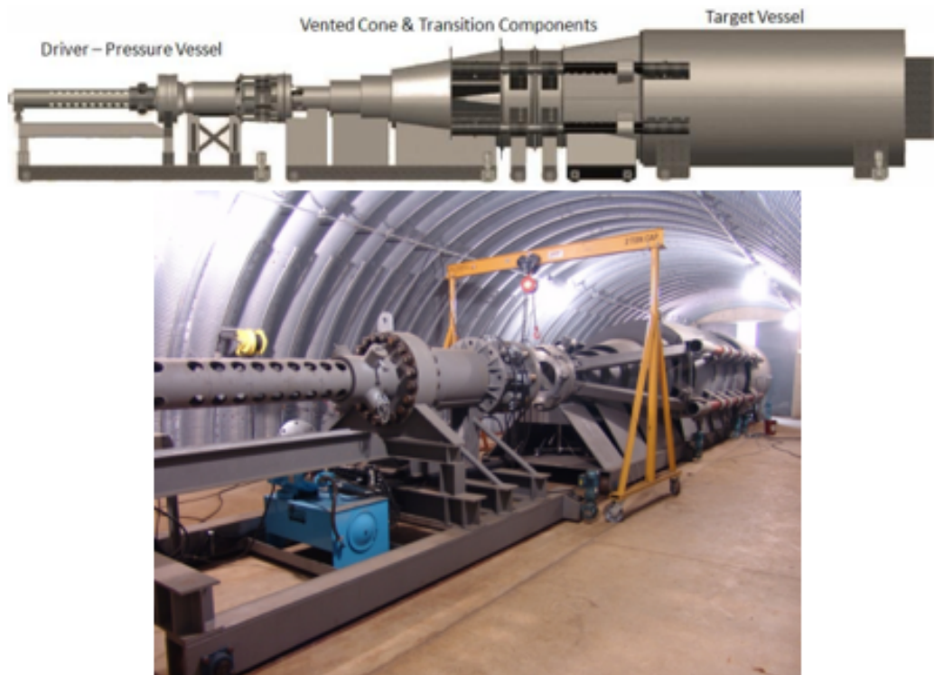
Figure 1- Blast Load Simulator (Top) Schematic (Bottom) Photograph
