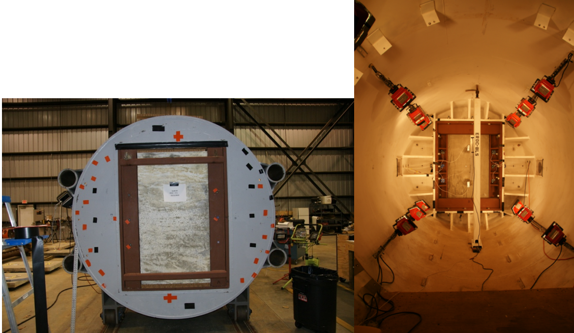
Figure 2- Slab Placement in the Blast Load Simulator (a) Viewed from the Blast Side, (b) Viewed from the Face Opposite the Blast Side
