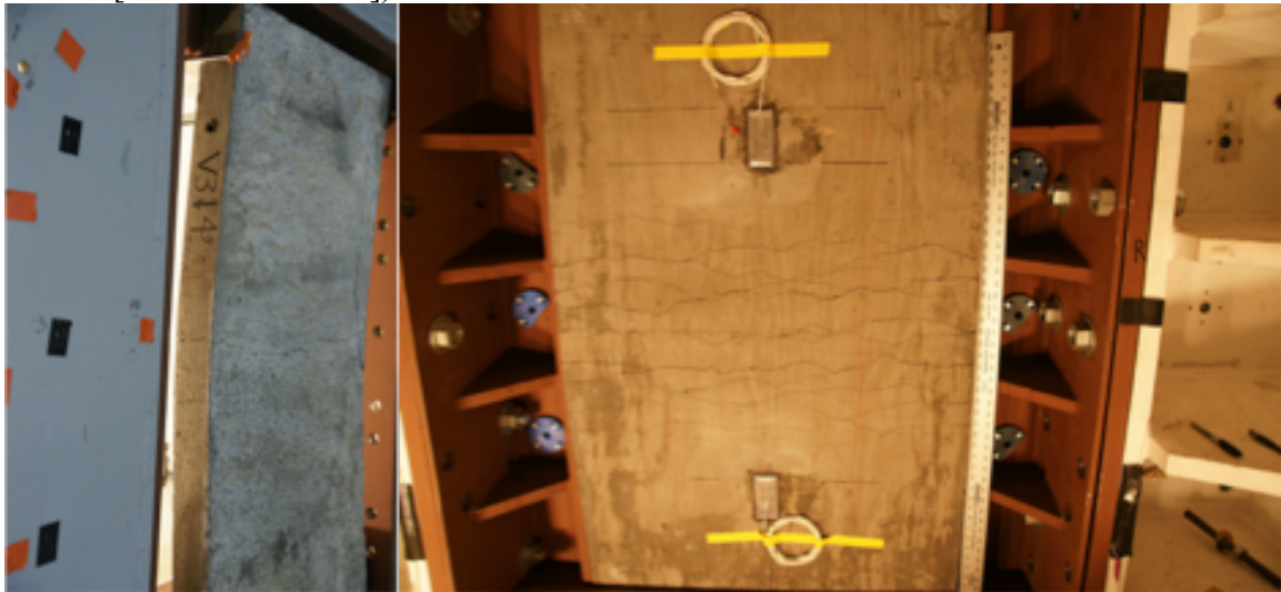
Figure 28- Damage to HSCV2 (4 in. [101.6 mm] Spacing; P = 49.2 psi [339.2 kPa]; I = 997.6 psi-msec [6878.2 kPa-msec]).
