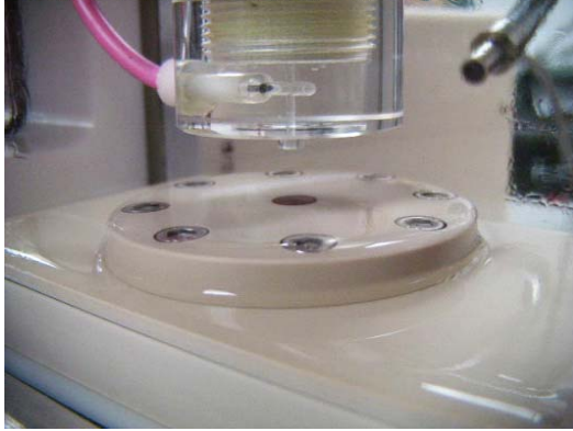
Acrylic nozzle D_i = 1\text{mm} , D_o = 4\text{mm} a 0.5\text{ cm}^2 smooth surface with flat cover
