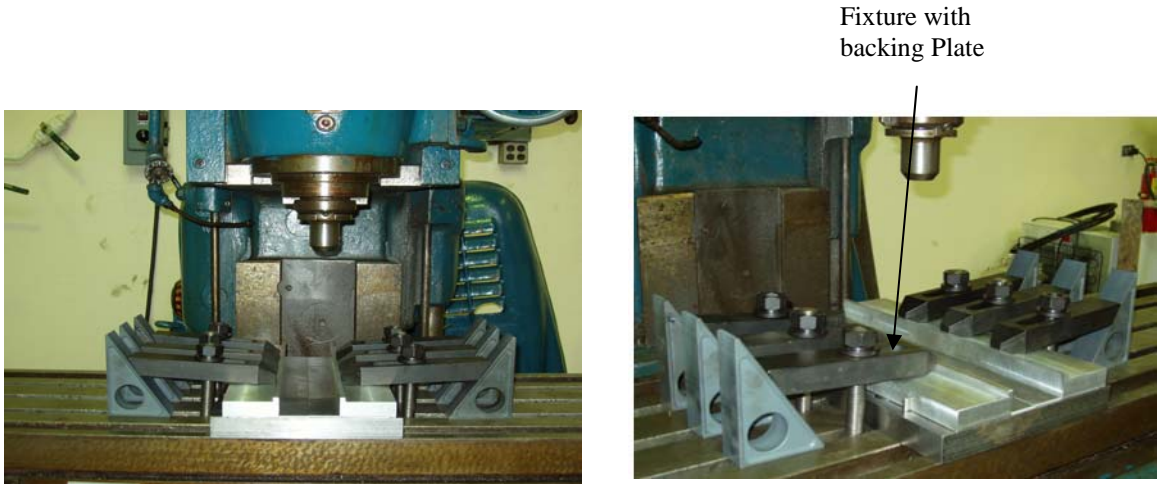
Figure 3.4 Adapted Milling Machine with fixture for Friction Stir Welding
