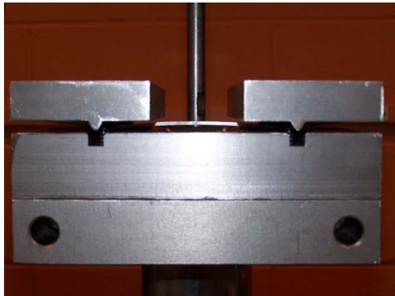
Figure 3.10 Tool Set Up of Stretch Forming Process
