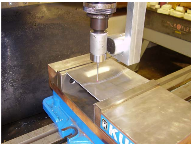
Figure 3.17 The Measurement of the Square Pan on the CMM.
