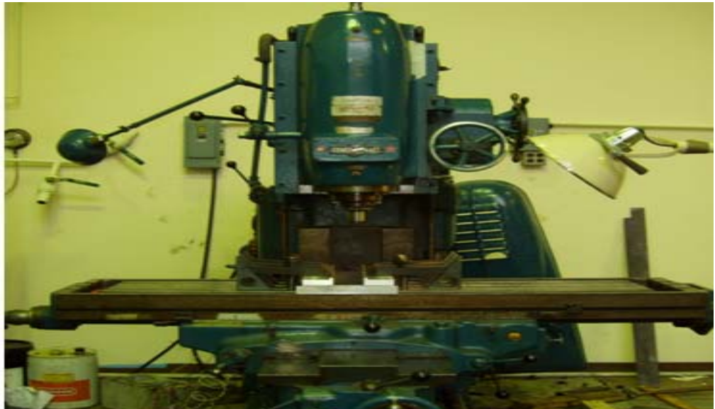
Figure 3.2 Adapted Milling Machine for Friction Stir Welding Process
