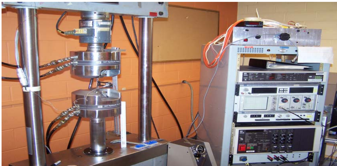
Figure 3.7 The hydraulic Linear Displacement Machine for Tensile Testing, with Extensometer in Place on the Clamped Sample.
