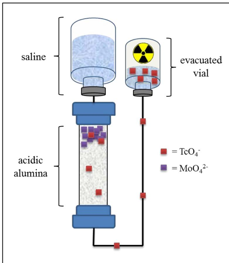
Figure 4-2. Scheme of a  $^{99m}\text{Tc}/^{99}\text{Mo}$  generator.
