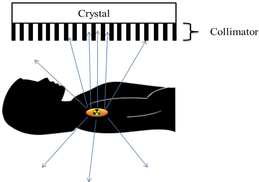
**Figure 4-1.** Illustration showing the use of a collimation system for SPECT imaging.
