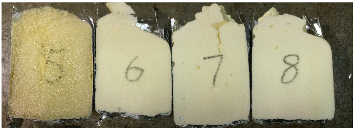
Figure 4-9 Longitudinal sections of foams with different surfactant loadings
