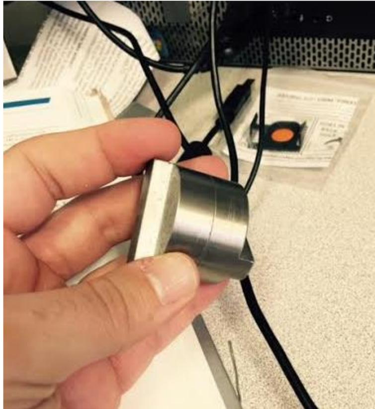
**Figure 9.4:** Unused molybdenum container
