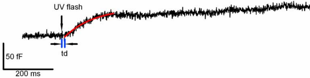
Fig. 3.8. Sample exponential fit to \Delta C_m elicited by photorelease of caged Ca^{2+} . The black trace represents a capacitance trace corresponding to the release of the HCSP. The red trace illustrates an exponential fit for the first 200 ms of capacitance change corresponding to the release of HCSP. For this sample trace, the fitted parameters are A_m = 46.6 fF, k = 8.35 s ^{-1} , T_d = 19.8 ms. (td: delay time between flash and exponential response).
