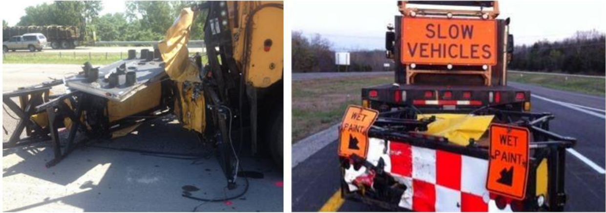
Figure 1.1.3 Aftermath of two separate mobile work zone TMA collisions
