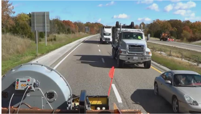
Figure 4.1.5.2 Example of sudden braking by silver car causing dump truck to quickly apply the brakes at DAS Actuated setup
