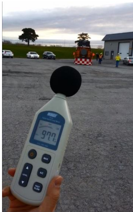
Figure 3.1.3.2 Sound level test while walking for DAS
