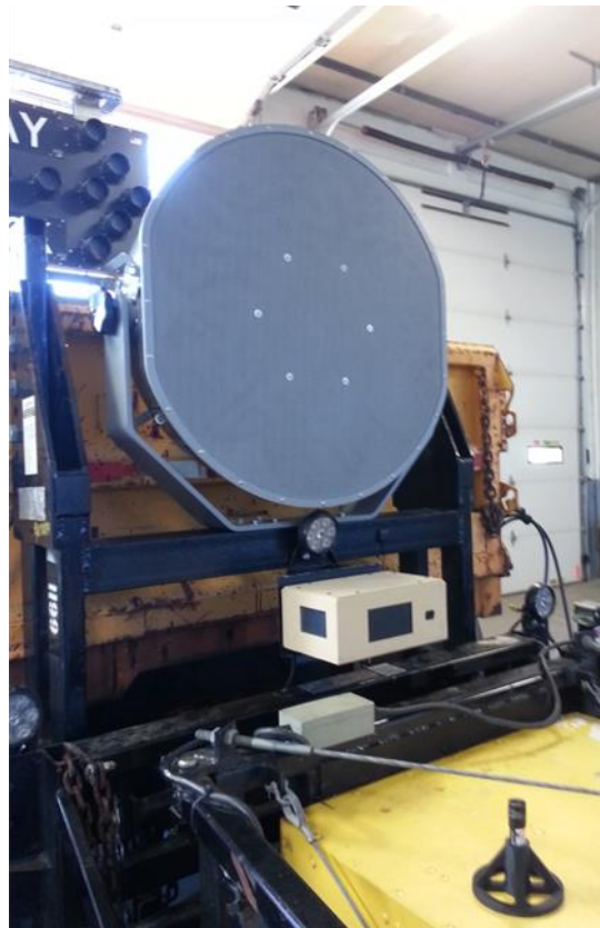
Figure 1.1.5 TMA truck with DAS unit
