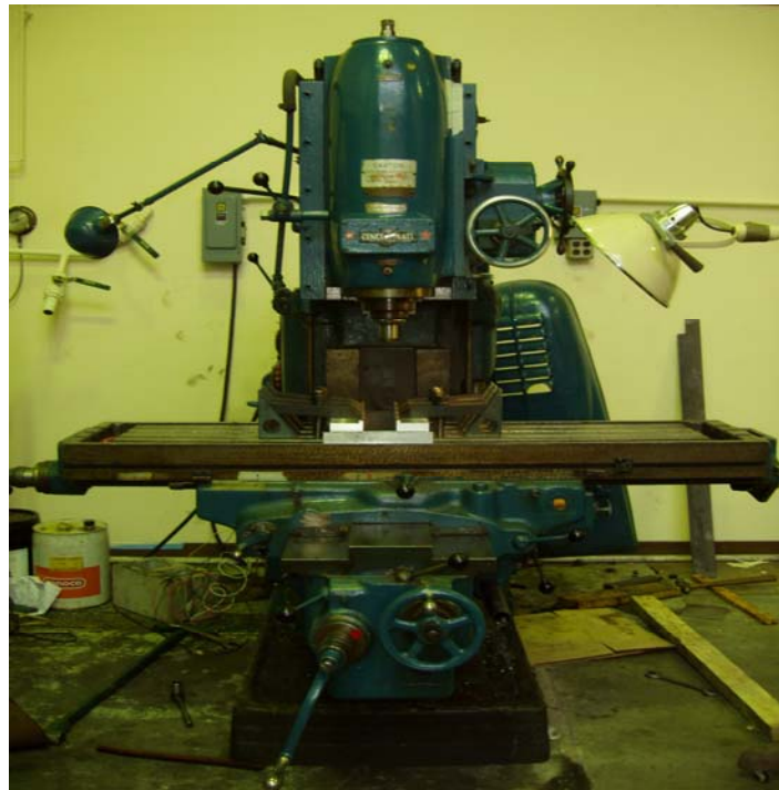
Figure 2-1 Cincinnati vertical milling machine transformed into a friction stir welded machine for research the picture shows the fixture designed for the machine to transform it into a FSW machine.
