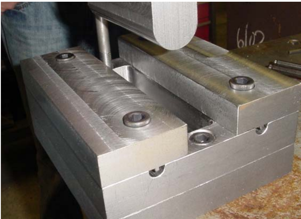
Figure 2-9 Close up view of stretch forming die figure shows the die set (base), top plates and the punch
