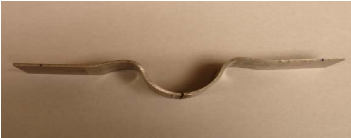
Figure 2-11 Specimen after the stretch forming of AA 2024-T3, the sample has formed to take the shape of the punch of the stretch forming die
