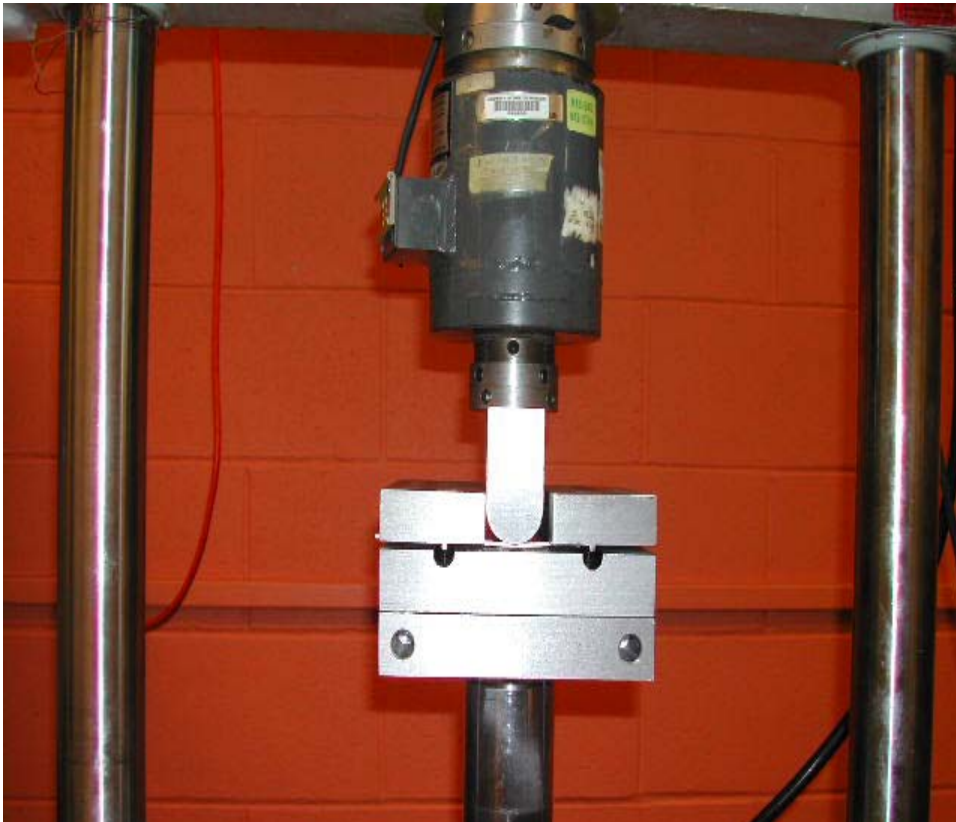
Figure 2-10 Experimental setup for the stretch forming process
