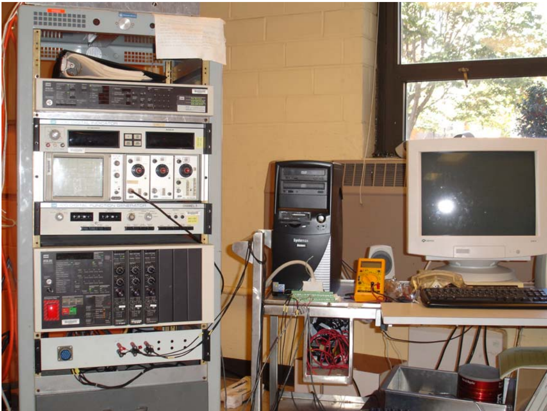
Figure 2-7 Data acquisition system for the MTS machine
