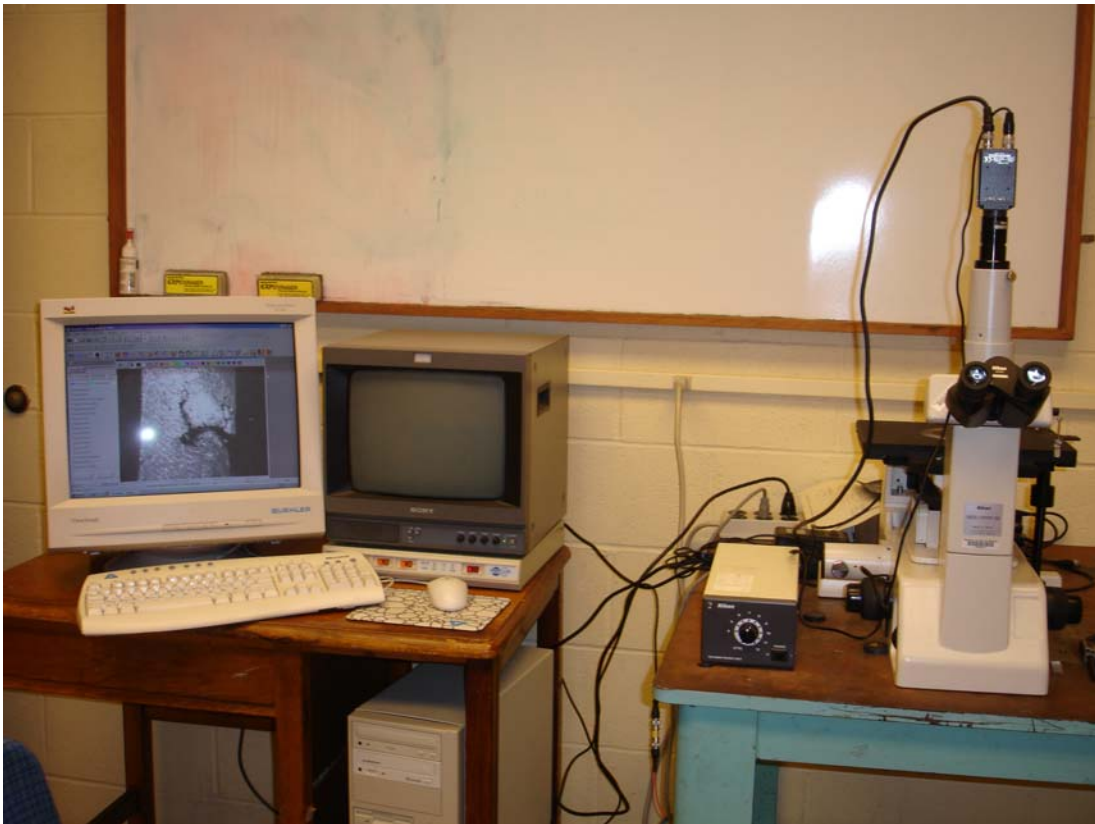
Figure 2-18 Optical microscope and the data acquisition computer used for the study of the microstructures
