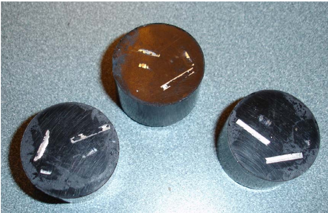
Figure 2-17 Samples mounted in phenolic powder on the automatic mounting press with some powder on the samples which can be removed by polishing
