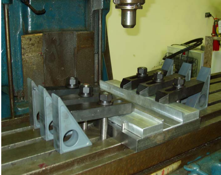
Figure 2-2 Fixture designed for transformed to transform conventional milling machine into a friction stir welding
