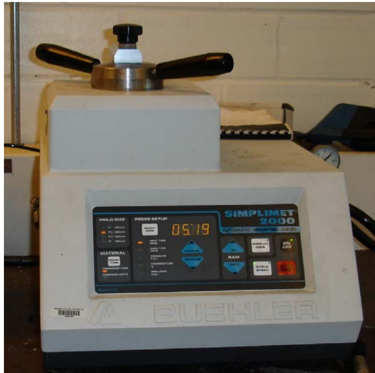
Figure 2-16 Buehler automatic mounting press used for mounting the samples for the microstructure study.
