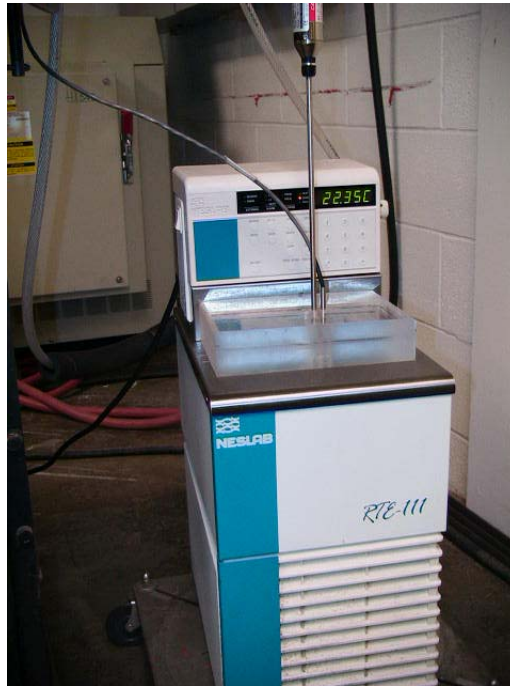
Fig. C1. Calibration of Thermistors using Kaye Intelligent RTD Temperature Probe.
