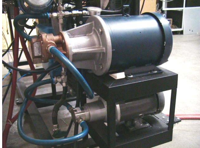
Fig. 13. Stacked 1-hp and 3-hp pumps for Unit Cell liquid loop.
