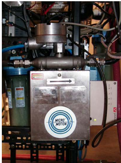
Fig. 14. Micro Motion® flow meter used for water flow measurement.
