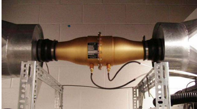
Fig. 28. Laminar Flow Element used for air volumetric flow rate measurements.
