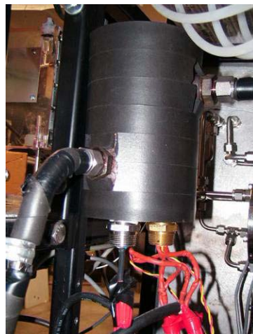
Fig. 15. Heating section of Unit Cell liquid loop.
