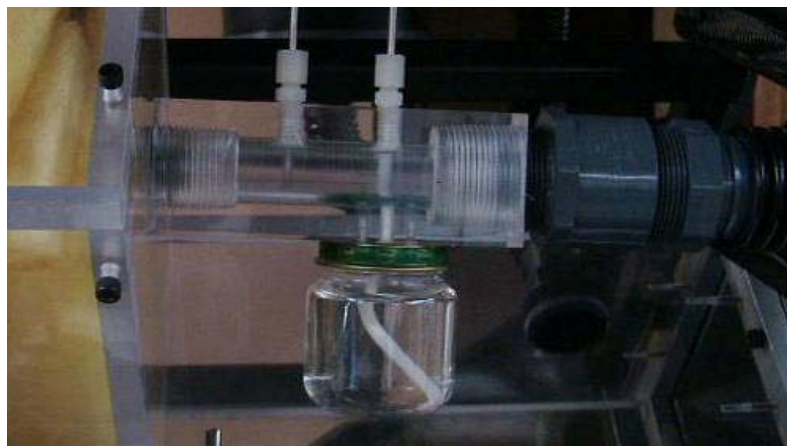
Fig. 19. Air dry and wet bulb temperature measurement system.
