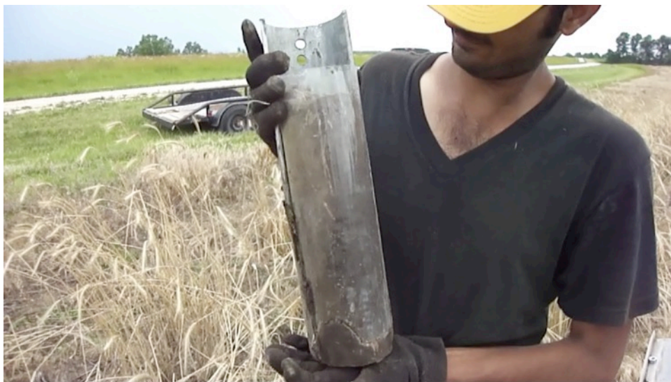
Figure 3.4. Collecting soil cores using a Giddings soil core sampler for the greenhouse study at Chariton County Soil Health Farm, Missouri.
