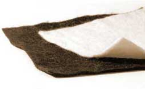
Figure 2-3. Example of Non-Woven Geotextile Fabrics (Monlux et al., 2000).
