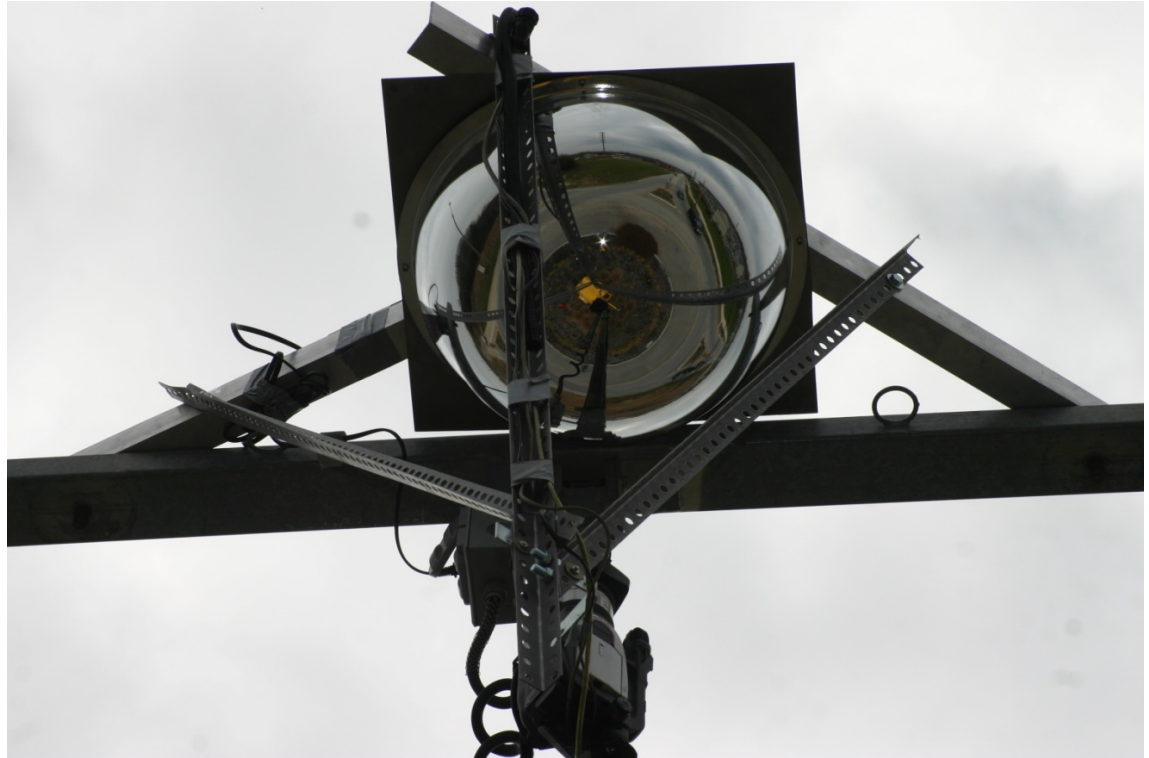
Figure 12: Close up of dome mirror and camera mounting bracket on the POST trailer
