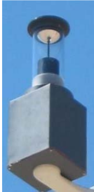
Figure 11: Remote Reality OmniAlert360 camera
