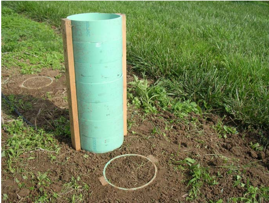
Figure 11. A soil cage tube assembly above ground (left) next to a buried tube (right). Each soil cage tube was filled with soil and allowed to settle for one month prior to adding the weevil larvae.
