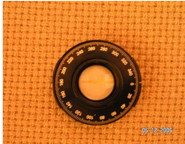
Figure 3-4. Rotating apparatus used for fiber alignment Raman measurements.
