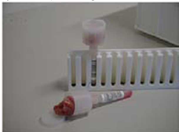
Figure 4. Example of specialized drip loss tube (manufactured and distributed by C. Christensen Laboratory, Denmark) and storage rack.
