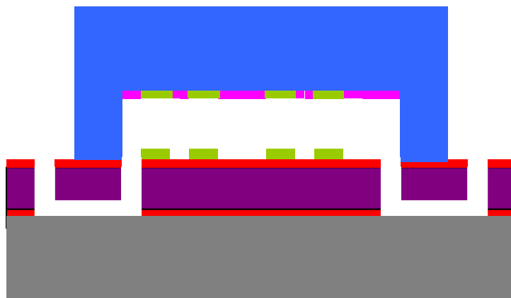
4.11h) Image showing the cross-section of the complete device after etching out the holes for inlet and outlet, removal of sacrificial layer and glass bonding.
