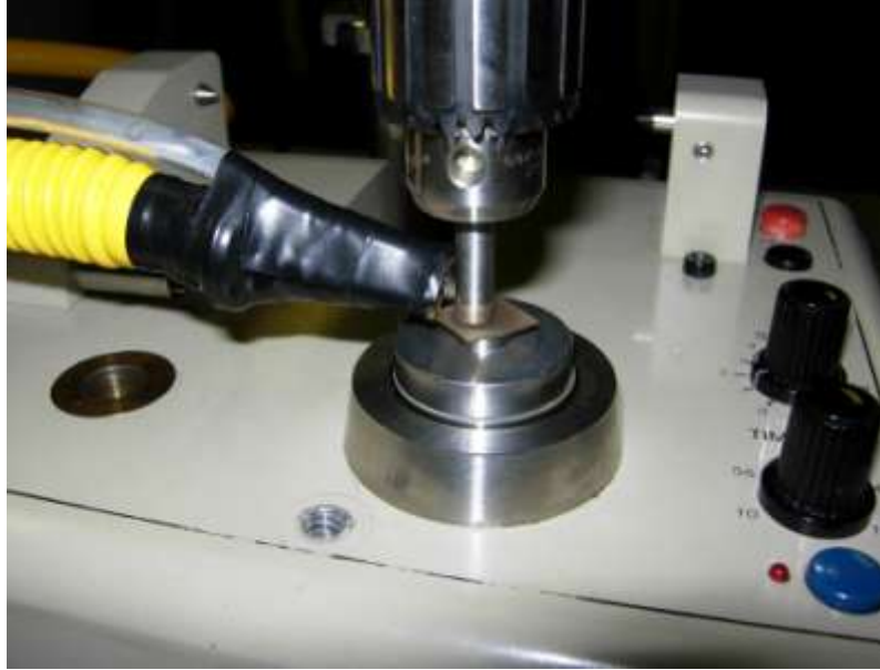
Figure 4.12 Initial grinding setup for conceptual testing.
