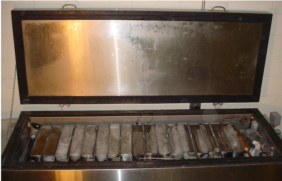
Figure 4-5: Freeze-thaw cabinet shown during thawing portion of a cycle
