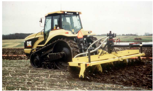
Figure 3. Liquid manure pumped from a manure storage facility is incorporated into the soil by rotating tines. This method reduces odors associated with surface application of manure.
