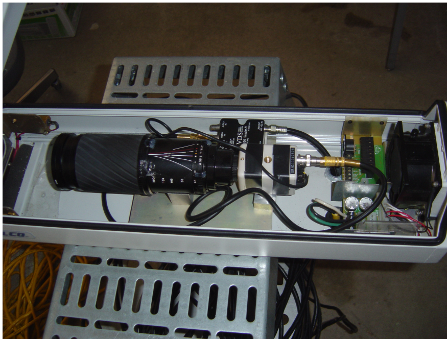
Figure 3.3: Image of the camera component of the RIS.
