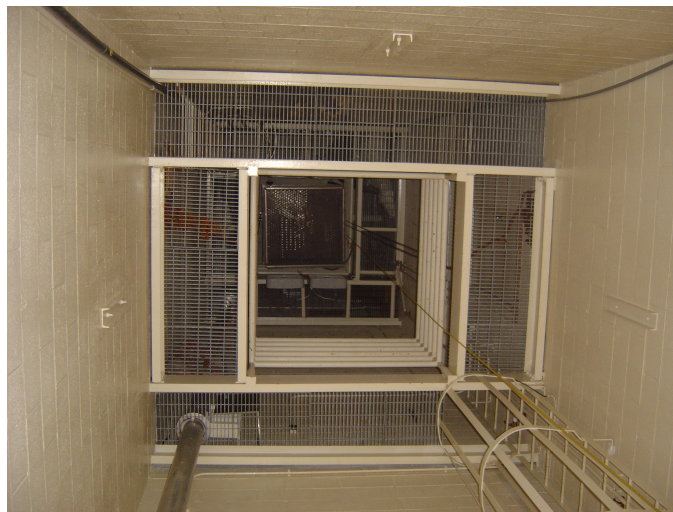
Figure 3.9: View looking upward showing the vertical extent of the indoor rainfall simulator located in the Hydrology Laboratory.
