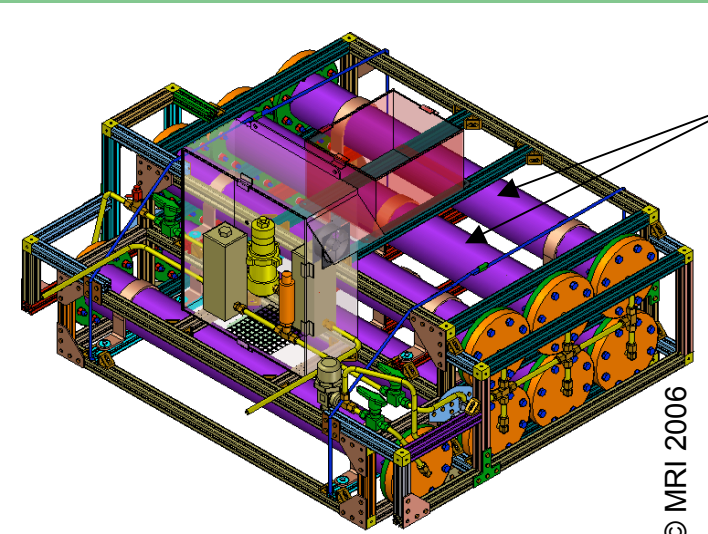
6 Al tubes holding 300 carbon briquettes
