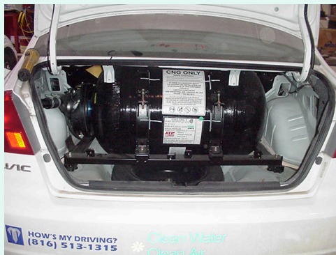
Current NG vehicle with high-pressure tank in trunk
