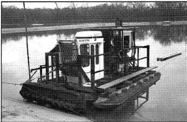
Figure 3. The horizontal auger on this dredge can be lowered to the bottom of the lagoon for biosolids removal.
