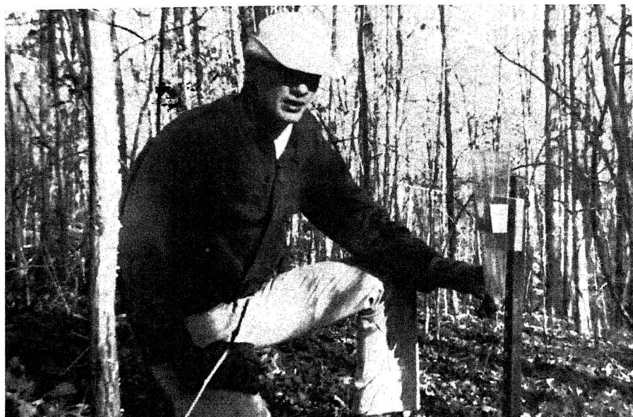
Fig. 2—Plastic rain gage used to measure throughfall on Gum Springs Watershed.
