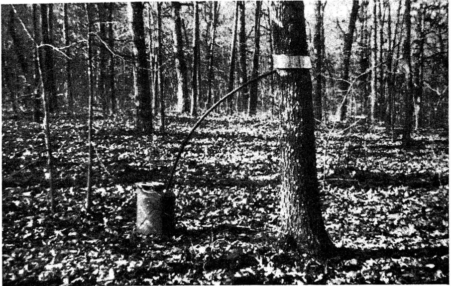
Fig. 4—Stemflow collar, hose, and collection container for tree on Gum Springs Watershed.
