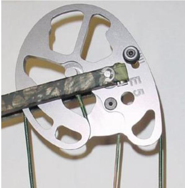
Figure 32 - Binary Cam; No Split-harness Connection to Limb [ www.bowtech.com ,2009]
