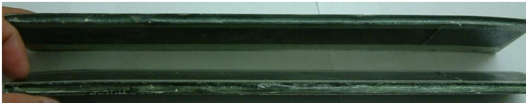
Figure 44 - Experiment 2; Visible Deformation in Sample #1 and #2 with Foam Core
