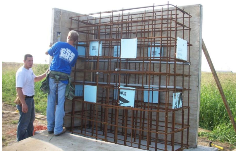
Figure 3.6 : Photograph showing the North face of the block with Styrofoam targets and Thermocouple Arrays in PVC tubes.
