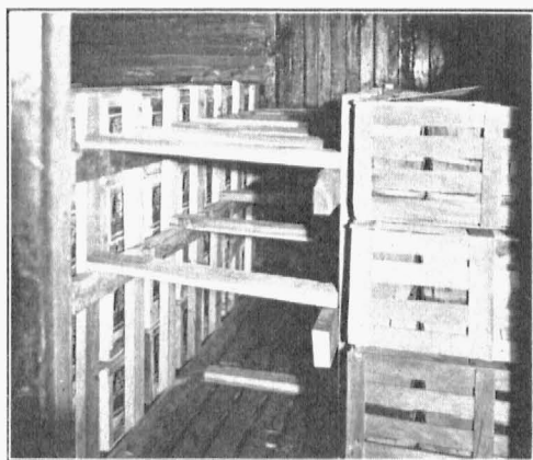
Fig. 6.—View from the refrigerator car door showing strawberry crates properly loaded, braced and the car ready to move to market.
