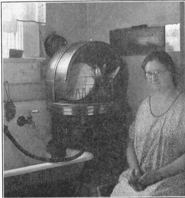
Fig. 4.—An electric dish washer saves much time and work on Farm 11. The hose is attached for running hot water into the bowl of the washer. A motor and pump below the bowl of the washer force water through a set of nozzles under the basket of dishes.
