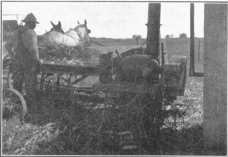
Fig. 9.—A 5 H. P. silo filling unit in use on Farm 35. The frame for mounting the motor on the cutter is not regular equipment.
