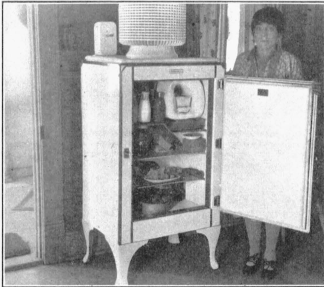
Fig. 19.—An electric refrigerator placed in the kitchen saves many steps on Farm 34. For the hottest month in 1928 it cost $1.93 (3c a KwH) to operate the refrigerator.
