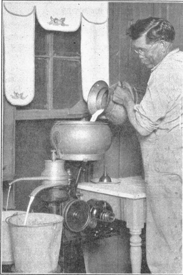
Fig. 3.—A motor driven cream separator used on Farm 2. At 10c a Kwh it costs less than \frac{1}{4} c a day to separate 14 gallons of milk.
