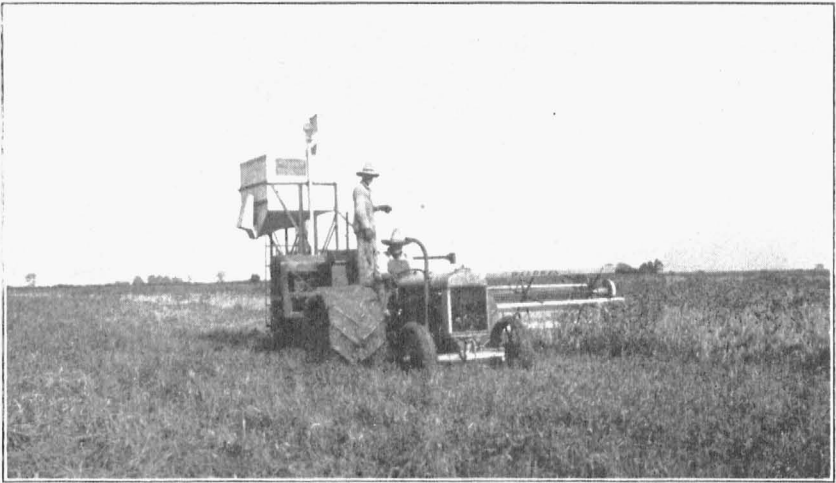
Fig. 6. Direct combining a field of wheat on a Carroll County farm. The principal advantage of combining over the binder-thresher method, is saving in time, labor and expenses.
