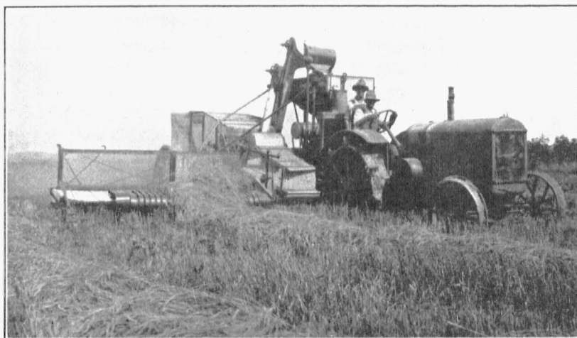
Fig. 5. Threshing wheat from the windrow on a Buchanan county farm. The windrow system enables a combine to harvest a larger acreage in a season.
