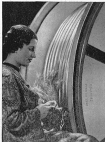
Every wire in every cable made at Western Electric receives many tests before it is acceptable for your service. Here is one of the final tests after the lead covering is applied.
