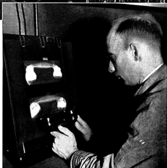
An unusual inspection, typical of Western Electric thoroughness. The operator has taken an X-ray picture of the telephone, to make sure its "innards" are all right.
